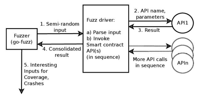
Figure 2: Fuzz Test Control Flow for One Cycle
