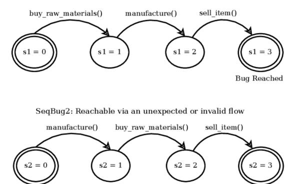
Figure 7: State machine representing API calling sequences to reach sequence bugs
